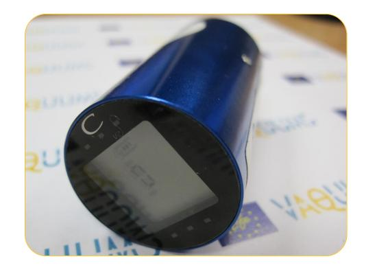
The CairClip  $O_3/NO_2$  is a lightweight, portable sensor for measuring ozone and nitrogen dioxide in ppb or  $\mu g/m^3$  in applications such as personal exposure and indoor and outdoor air quality monitoring. To calculate the concentration of ozone, it needs to be combined with the CairPol CairClip  $NO_2$  sensor, since nitrogen dioxide concentration needs to be subtracted from the measurements of this sensor.
